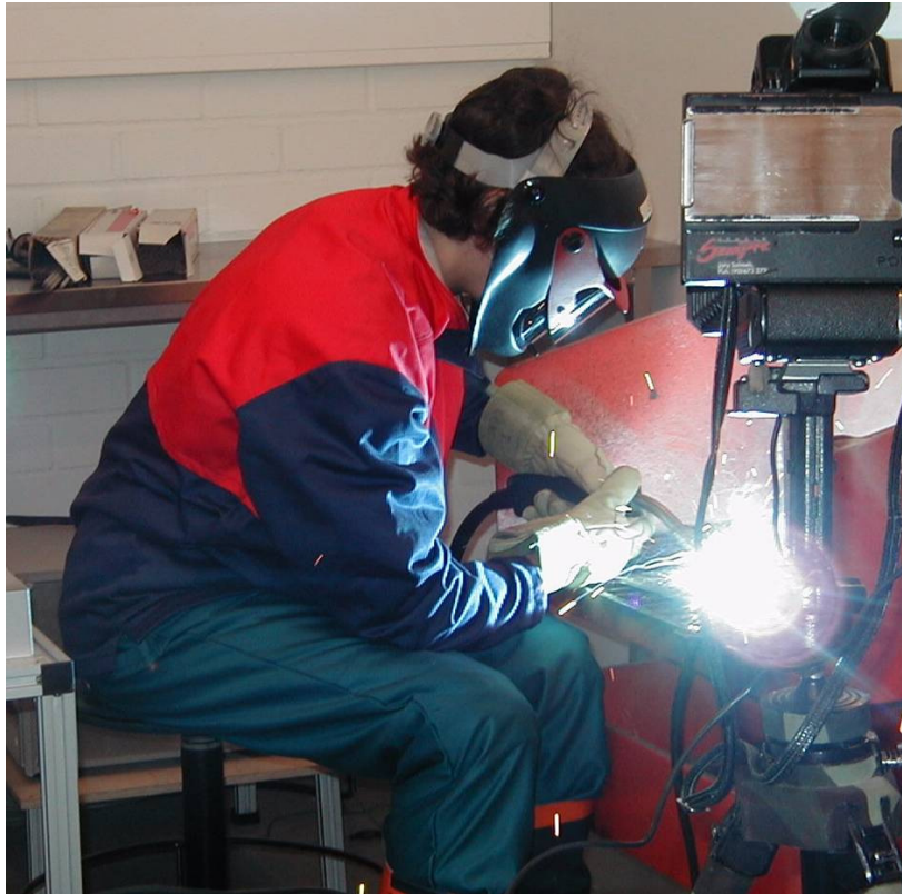
Figure 11. Welder with appropriate personal protective equipment for the eye and skin (Photograph courtesy of Finnish Institute of Occupational Health)
