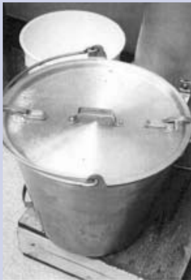
Many metal buckets have metal lids with clasps and a tight seal to prevent splashing.
